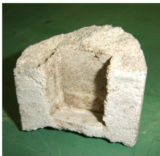
Figure 9. Gypsum mould obtained by lost-wax pattern by capillary moulding by Variant 3; compound of the “dry mass” G/S = 1/2,5 weigh part
