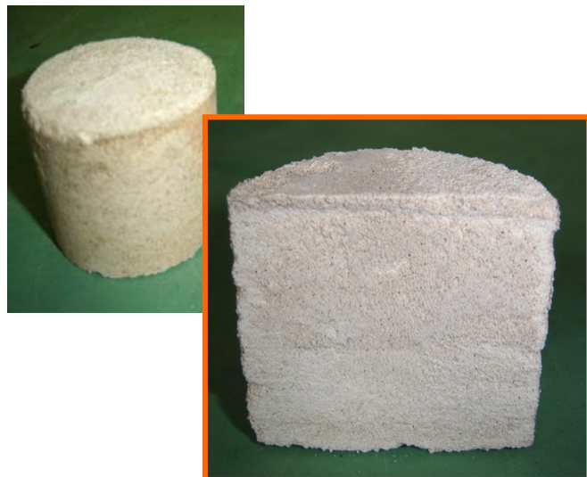
Figure 6. A view and a longitudinal cross-section of a sample, obtained by Variant 3; weigh ratio G/W = 1/2
