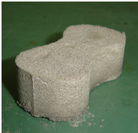
Figure 3. Sample for determining of the tensile strength R_r
